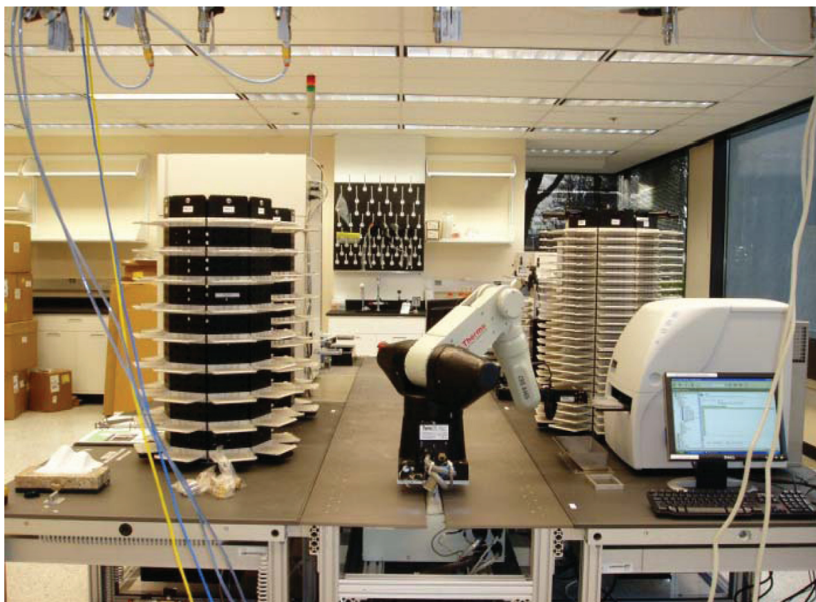
Figure 2. Automated high throughput assay robotic system for pathway readouts: Automation processes for reagent addition, compound dispense and assay detection enable signaling panel approaches for compound evaluation in multiple cell lines.
