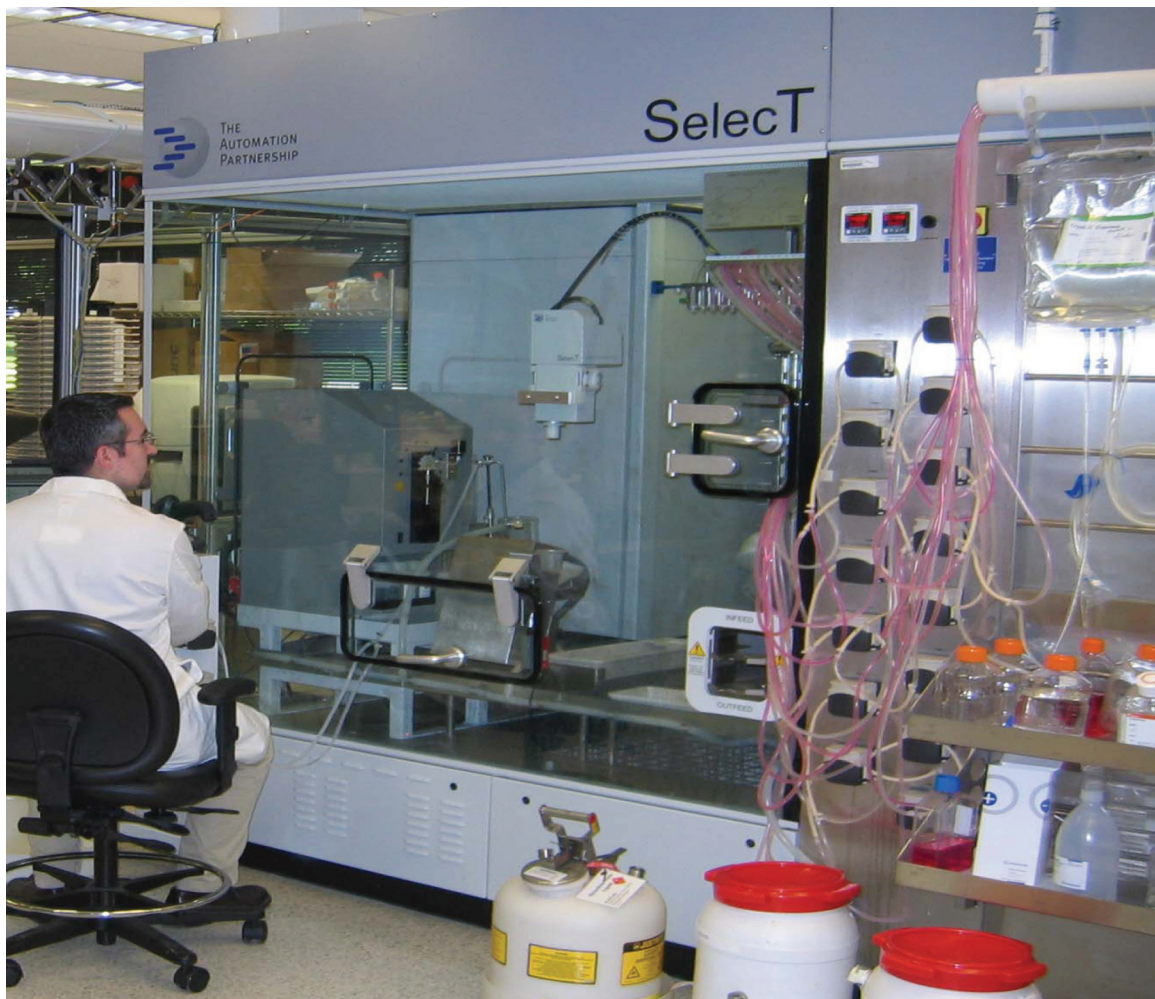
Figure 1. Automated cell culture system—SelectT: Cell culture automation with capacity to process more than 60 cell lines and up to 175 flasks enabled the cell line panel approach for signaling readouts. Cells can also be plated into 384 assay plates using this technology platform.
