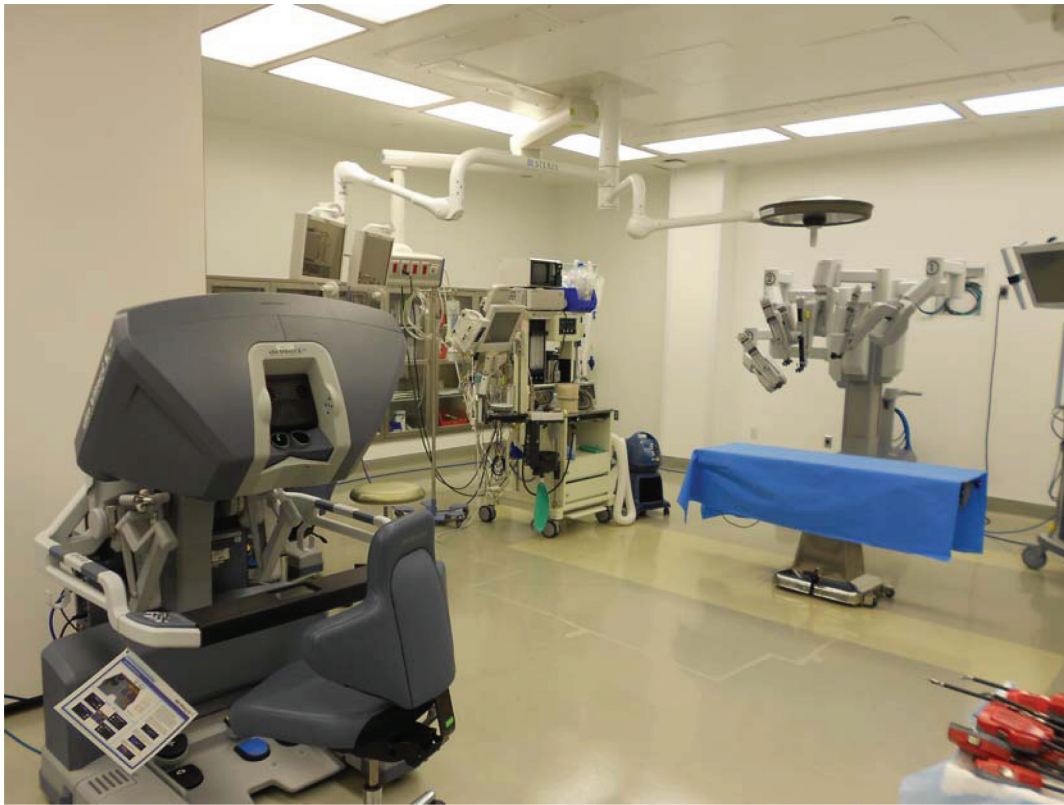
Figure 1. The Da Vinci Surgical System has an ergonomic console that remotely controls the various arms of the actual robotic unit performing the surgery.
