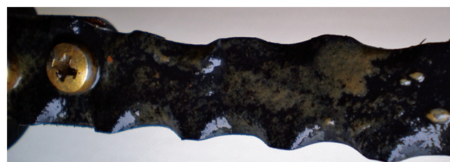
Figure 2. Black polypropylene substrate with associated biofilm. Biofilm appears as rusty orange/brown depositions on the surface of the plastic.
