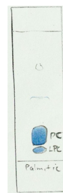
Figure 6. Thin layer chromatography of dipalmitoyl phosphatidylcholine with traces of its lyso analog.
