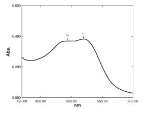
Figure 3. Absorption spectra of the complex formed through reaction of 1.8  $\mu gm^{l-1}$  Moxifloxacin HCl with 2,2' bipyridyl and FeCl<sub>3</sub>.
