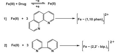
Figure 1. Reactions of moxifloxacin HCl with 1,10 (o-phen) and 2, 2'(bipy).
