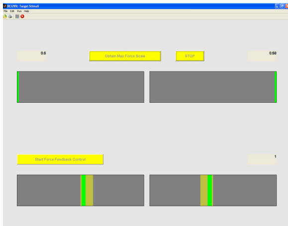
Figure 2. The screenshot of the home-made MATLAB-based paradigm for visual target tracking. Subject was asked to squeeze his/her fingers to the center of the track to measure the maximum force (upper part). Then subject performed repeated task: tracking the yellow target by the feedback squeezing force to make the narrow green inside the brown bar (lower part).
