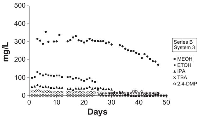
Figure 7 Series B System 3 alcohol concentration with time. 7.5 g dry AC, 100 g NASA GW, 0.6 g NASA soil, 500 µl Lactate/alcohol spike.
