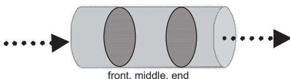
**Figure 2.** Schematic of smaller activated carbon column, showing three sampling sections for mass extraction.
