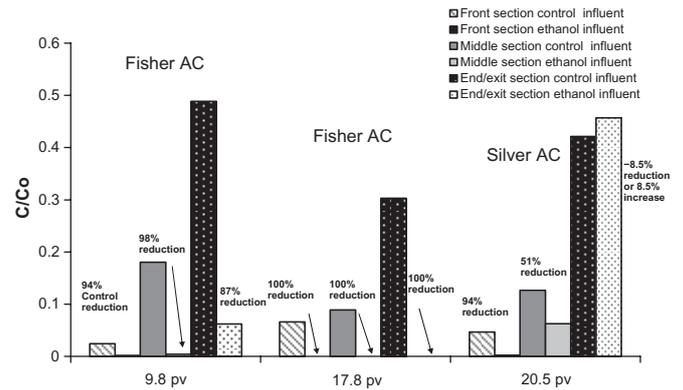
**Figure 11.** C/C<sub>0</sub> comparison of ethanol mass remaining on Fisher AC and silver-impregnated AC after specified number of pore volumes. Control signifies flushed with groundwater only.
