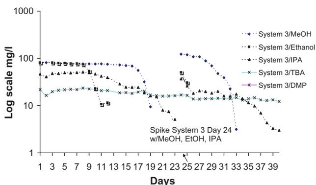
**Figure 4.** Series A System 3 spiked Day 24, alcohol concentration as function of time.
