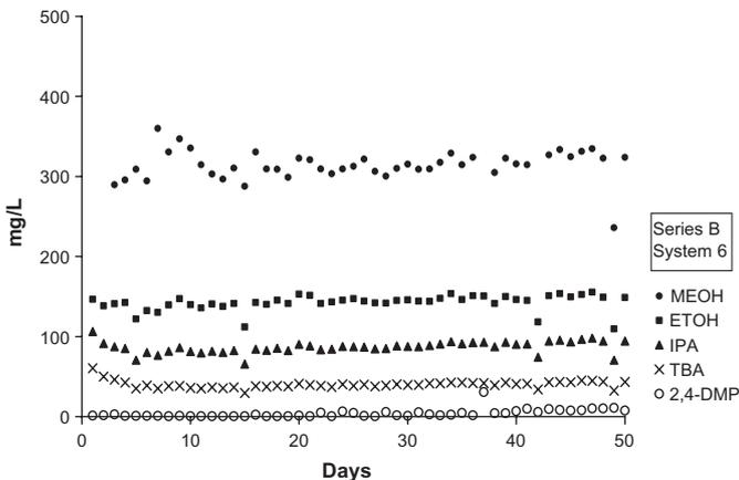
Figure 8. Series B System 6 alcohol concentration with time. 7.5 g silver AC, 100 g NASA GW, 0.6 g NASA soil, 500 µl lactate., alcohol spike.
