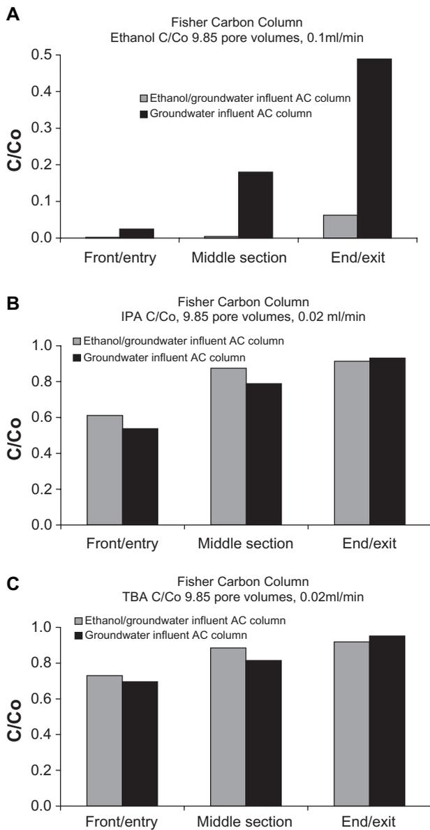
**Figure 10.** C/C<sub>0</sub> comparison of alcohol fractions according to column section, 9.85 pore volumes, 0.02 mL/min. A) Ethanol. B) Isopropanol. C) Tert-butyl alcohol.
