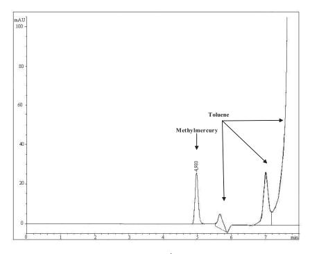
Figure 4. Chromatogram of MeHgCl standard using a 25-cm Zorbax CN<sup>-1</sup> column.
