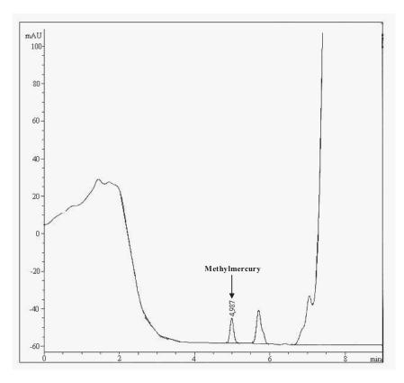
**Figure 5.** Chromatogram of the locality Frontera Peña—Orinoco contaminated with methilmercury standard of 50 ng.ml<sup>-1</sup>, in a proportion 1:1. Retention time for MeHg = 4.99 minutes.
